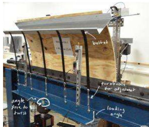
(b) photo during test of plywood sheathed specimen
