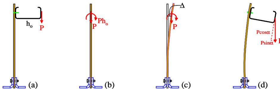
Figure 10: Large deformation effects in cantilever test (a) test (b) sheathing with forces (c)  $P-\Delta$  moment (d) load direction
