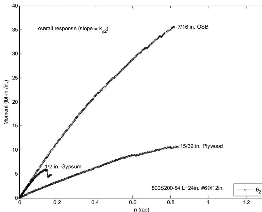
Figure 5: Typical moment-rotation results for overall stiffness (1 lbf = 4.448 N)
