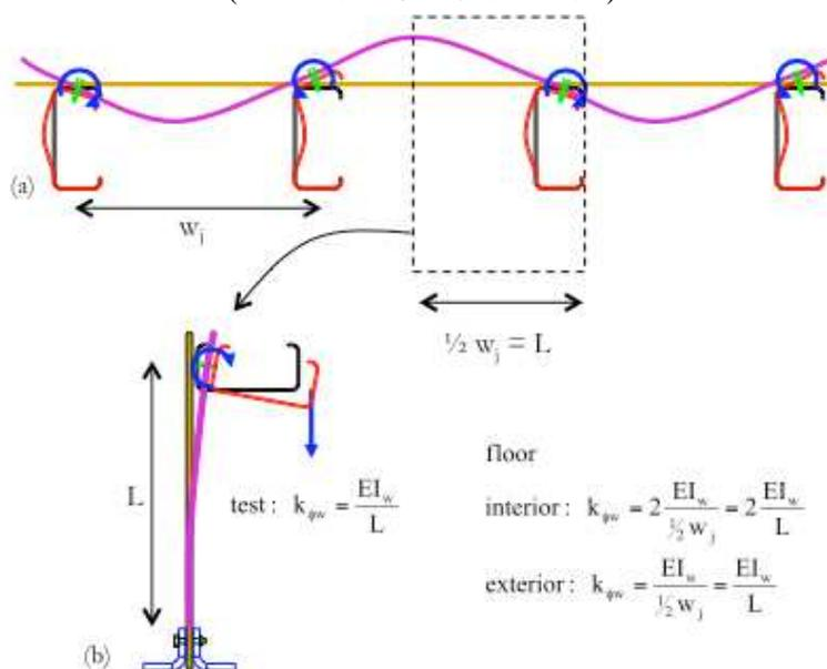
Figure 8: Sheathing stiffness for interior and exterior joists and comparison to conducted tests
