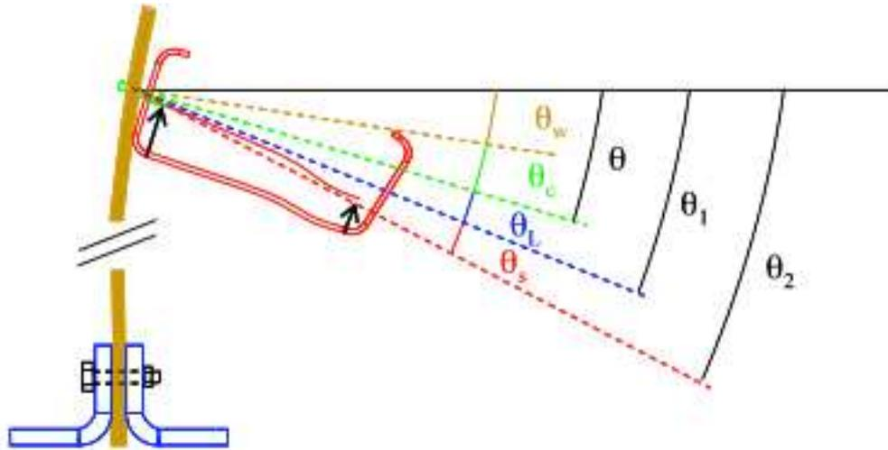
Figure 3: Breakdown of rotation at the joist-sheathing juncture
