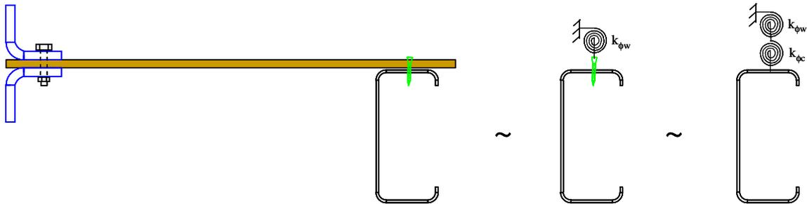
Figure 4: Illustration of rotational springs for sheathing and fastener
