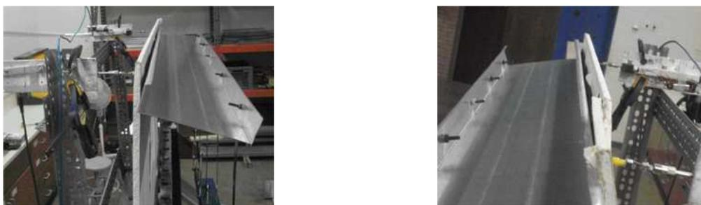
(a) large separation between joist and gypsum board      (b) pull-through failure and fracture of gypsum board
