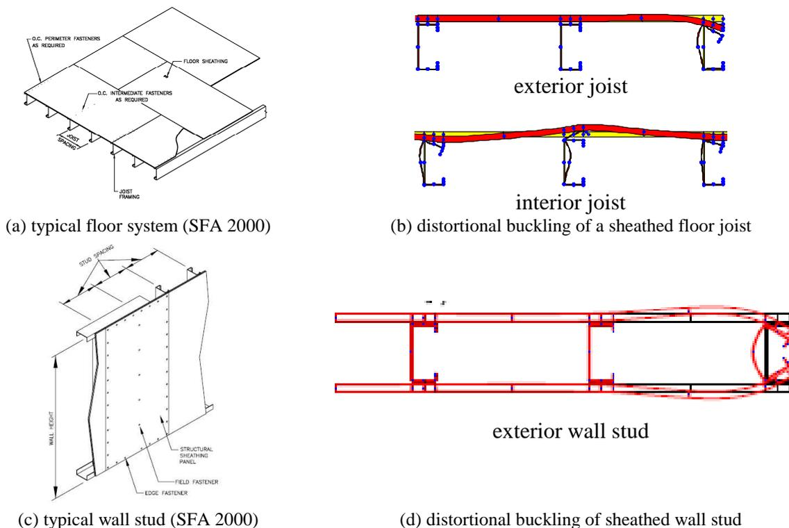
Figure 1: Distortional buckling of a floor system, sheathing provides rotational restraint
