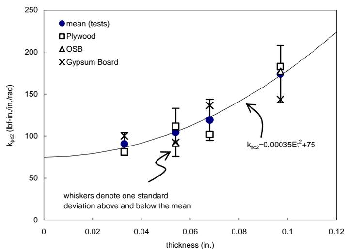
Figure 9: Connection rotational stiffness as a function of joist thickness
