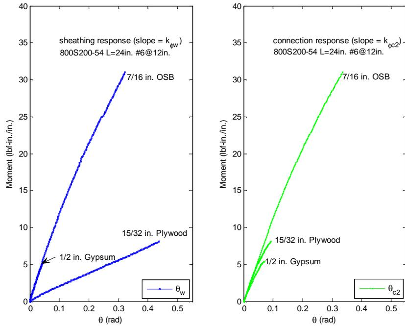
Figure 6: Typical moment-rotation results for sheathing & connection stiffness (11bf = 4.45N)
